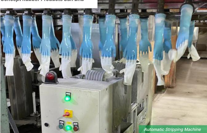
Concept Rubber Products Sdn Bhd, a manufacturer of latex examination gloves, male external catheters, and custom-dipped rubber products, has modernised its production process with the help of the Fund for Automation and Green Technology (FAGT) by MRC. The company has implemented an automatic stripping process to enhance efficiency, reduce labour dependency, and improve product quality.
